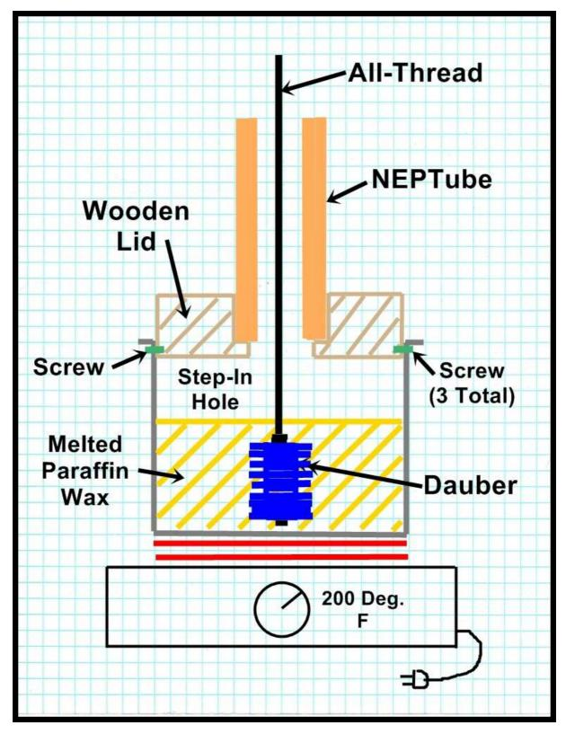
Here is a simple diagram of my original tube waxing apparatus:
