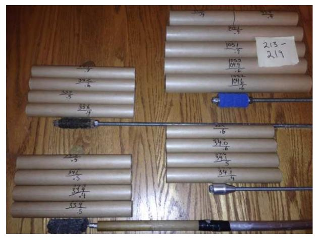
The numbers on the tubes indicate the weights of the tube before and after waxing, and the difference in grams. There is not much difference in the amount of wax applied with the different daubers. For a 1-pound tube 7 ½" long, about half a gram of paraffin is applied. The dauber on the upper left is my original one, made by wrapping jute around a threaded rod and putting nuts on the ends.
