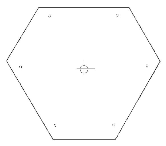
The following template can be printed and traced onto the material you are using for a hub. The small wire holes around the edge should be 1/16" dia, while the center hole depends on your your method of mounting the wheel. The method described in this article calls for a 3/8" dia. center hole.
